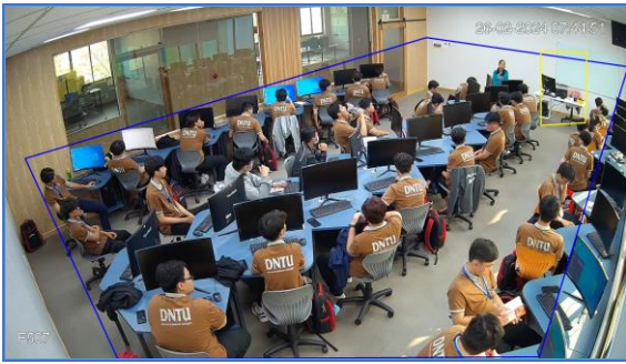
Figure 4. Description of counting areas. The blue line represents the polygonal counting area for counting students, while the yellow line represents the rectangular area designated for the instructor.
