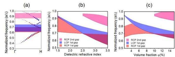
**Figure 2:** Band Structure and Gap Analysis of the Hybrid Metal-Dielectric Double Gyroid
