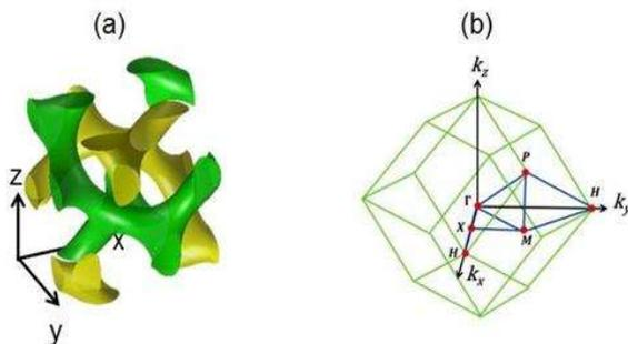
**Figure. 1** (a) The perspective view of a unit cell of metal/ dielectric DG with volume fraction = 20%. (b) The first Brillouin zone of DG (Chernow et al. 2021).
