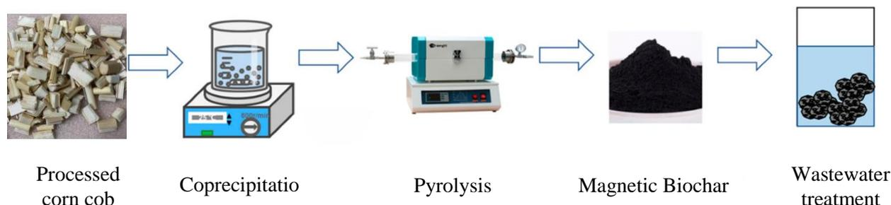
**Figure 1.** Process for synthesizing magnetic biochar
